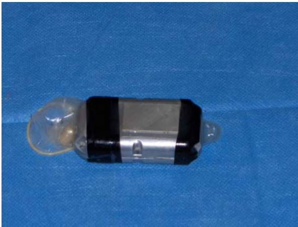
Fig. 3 Implant Case With Patch Antenna Enclosed in Latex Bag
